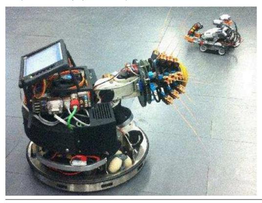
A new robotic system based on the Etruscan pygmy shrew can navigate by using tactile whisker sensors to build up a probabilistic map of its environment.
